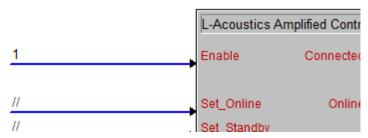
It is possible to use the standard "1" signal on all digital inputs of the module, especially on the **Enable** input. This will have the effect to instantly connect the module at program startup (for **Enable** input), or send the associated command as soon as the module connection is established (for other digital inputs).
